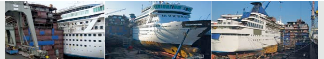
The construction of new luxury liners takes several years which is why shipping companies prefer to elongate their ships.
