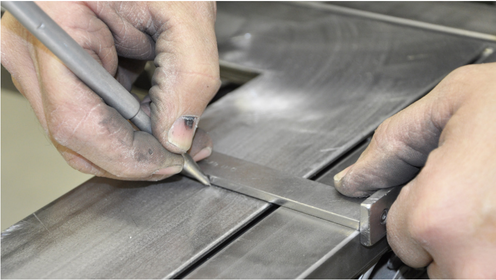
Marking by the means of a scribe and try square.
