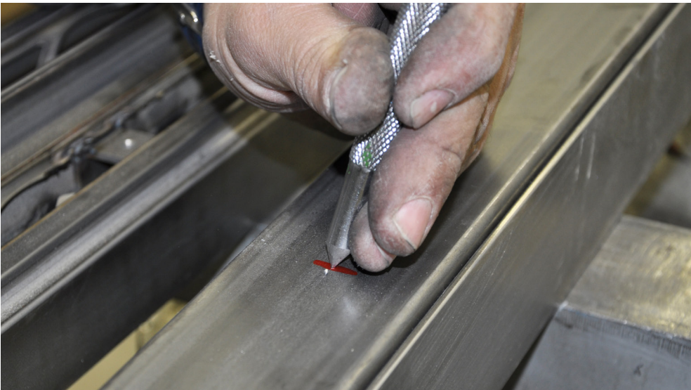
Punch setting by the means of a centre punch and hammer.
