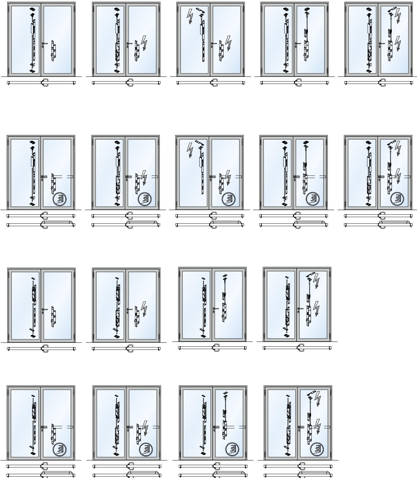
**Übersicht Beschlageinbau****Disposition de la quincaillerie****Placement of fittings**
