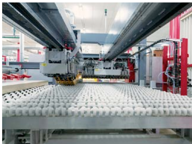
The machine table, which was treated by STI | Hartchrom for the Schelling panel cutting plant, has now been installed at Piatti.
